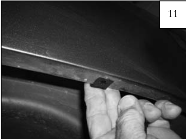
Center a supplied Clip (NU1-0007) over the upper two marks made in Step 9. Clips may need to be adjusted to align with holes in flare. Note: The raised collar on the Clip should face upward into the interior of the fender.
