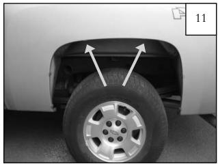
Slide a supplied Clip (CL1-0022) over top two factory holes. Clips may need to be adjusted to align with holes in flare. Note: Some vehicles with inner splash sheild will need to remove factory fasteners in indicated locations before installing the clips.
