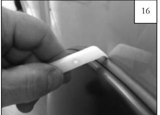
Using supplied Edge Trim Tool (ET1-0001), seat edge trim against vehicle by hooking curved end under edge trim at one end of flare. Next, slide around outer edge of flare to the other end.
