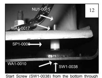
the Washer (WA1-0010) and into flare. Install Spacer (SP1-0008) between flare and sheet metal. Slide a Washer (WA1-0017) then a Nut (NU1-0015) over the end of the Screw (SW1-0038).
