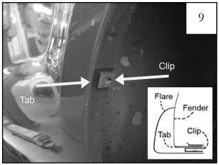
Install a Clip (CL1-0005) over each of the Tab (MT1-0014) installed in Step 8.
