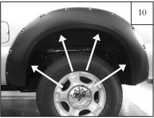
Position flare on fender and, starting with the two top holes, install Screws (SW1-0050) through holes in flare and into clips with a #2 Phillips screwdriver.
