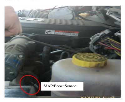
**6**) Unplug the MAP sensor and Plug in the Female plug from the module into the sensor
