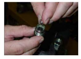
8) Remove the spring and insert the three shims as shown above
