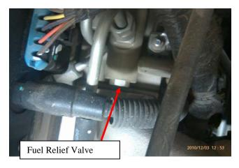
5)Use an 18mm wrench to remove fuel relief valve
