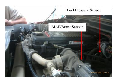
NOTE: If you do not see your MAP Sensor located where indicated on the picture above, we have seen some models with the MAP Sensor located where indicated on the picture below.
