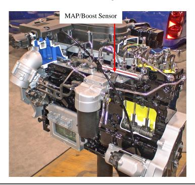
1) Locate Fuel Pressure Sensor on the drivers side of the engine
