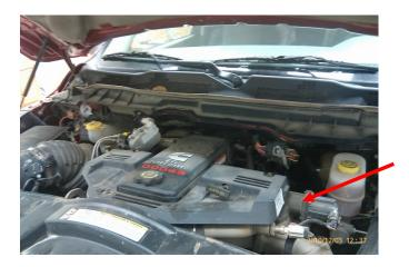
2) Using an 11mm wrench remove the 2 clamps holding the EGR tube that crosses in front of the valve cover.
