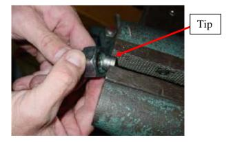
Note: Be careful to hold end of relief valve it is spring loaded and you don't want to lose any part. There is a small pin located in Tip behind the washer with three holes in it. Don't lose it, the truck will not run without it.
