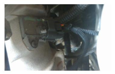
7) Plug the Stock Cummins MAP sensor connector into the Male Map sensor plug on the module harness
