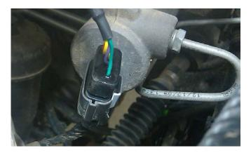
**8)** Route Switch through firewall and plug into module as shown below
