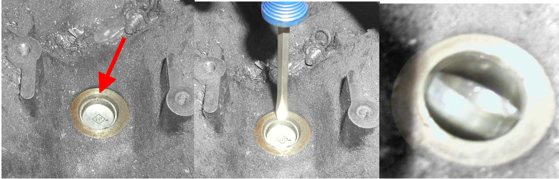
Figure 14 - Freeze Plug Removal
