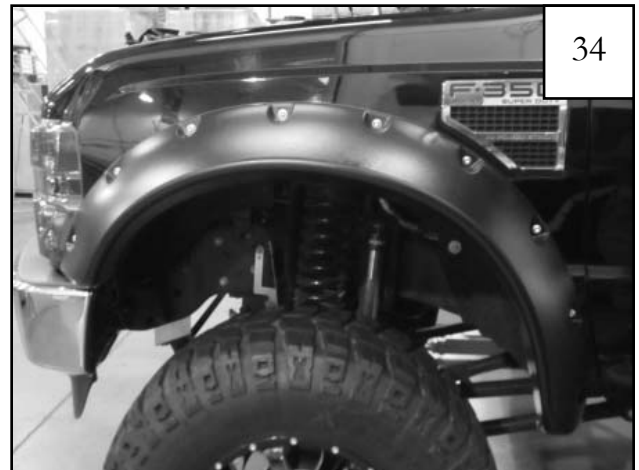
Completed front flare installation.
