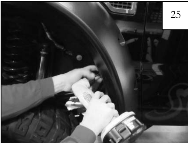
Install screw (SW1-0056) into holes drilled in previous step. Tighten ALL screws installed in Steps 23 & 24 to ensure proper alignment of flare for pocket hardware installation.
