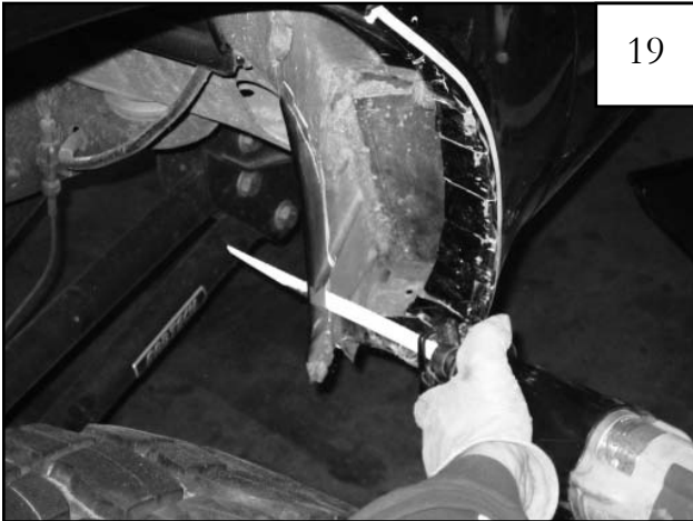
Using a Sawsall, cut along reference line.
