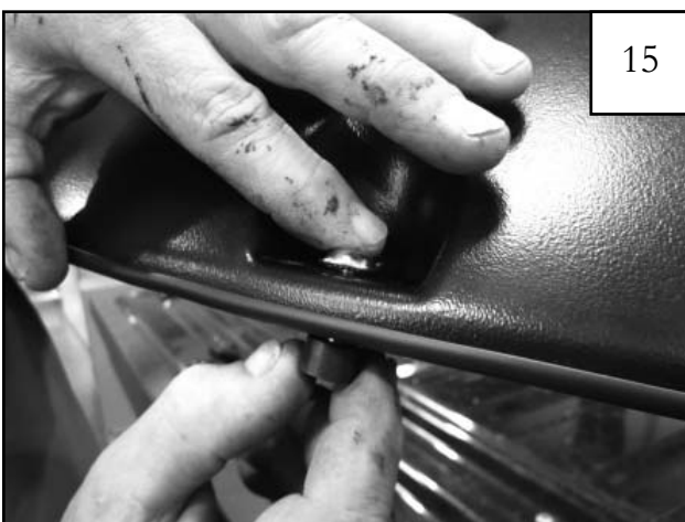
Thread bolt (SW1-0045) through pocket hole in flare then install spacer (SP1-0009) over end of bolt. Hand tighten spacer on bolt until snug near flare plastic.
