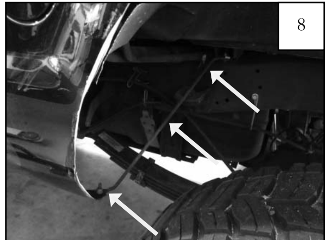
When cutting, be aware of support rod behind front side of wheel well. Angle blade inward to avoid cutting it.
