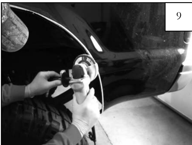
Using a grinder, debur cut edges.
