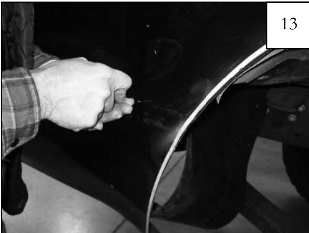
Using marks made with scratch awl as a guide, score the sheet metal with a center punch prior to drilling.
