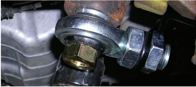
Idler arm bracket installed
