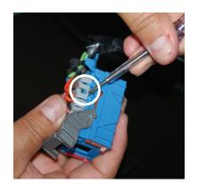
**STEP 15** Fully insert pin into the J3 terminal, #6 pin.
