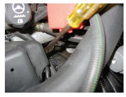
**STEP 8**Access the computer terminals. Locate terminal # 71. Disconnect the black plastic cover from the computer. Loosen clips located in the front and in the back.
