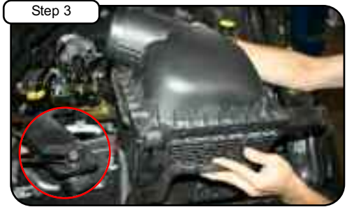
Step 3 Disconnect air temp & MAF sensor. Loosen 10mm nut holding in front of air box using wrench or socket. Lift up and pull OE air box out of vehicle.
