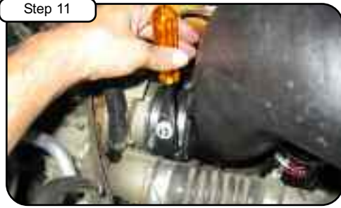
Step 11 Tighten turbo clamps using 5/16" nut driver. Re-connect crank case line into tube with grommet.
