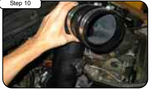
Step 10 Install hi-temp & hump coupler with clamps provided to tube. Now install tube into vehicle. Do not tighten!
