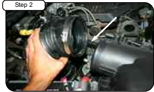
Step 2 With 5/16" nut driver loosen clamps on OE tube at turbo/air box and remove. Loosen clamp at turbo and disconnect crank case line with pliers. Remove tube.
