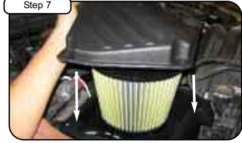
Step 7 Install air filter to cover housing, tighten using 5/16" nut driver. Place cover to bottom of housing and set to position.
