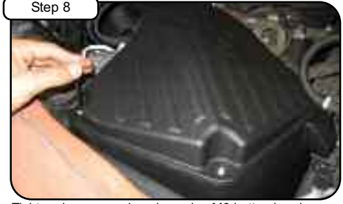
Step 8 Tighten down cover housing using M6 button head screws and wavy washers.
