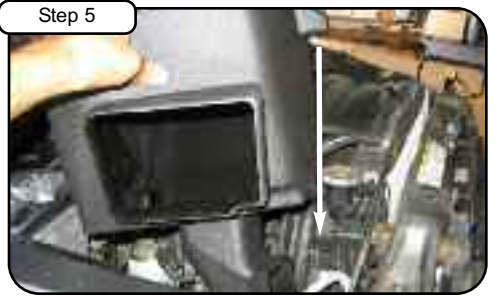
Step 5 With screws provided (see step 6), install housing into vehicle. Make sure housing tab mounts up to bracket "D" from step 4.
