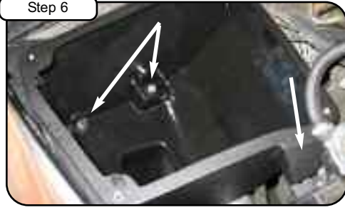
Step 6 With 3/8" screws/nuts and washers provided install bottom of housing to factory position. Tighten using 9/16" wrench or socket. Use M6 screw/nut/washers & wavy washer and tighten housing to bracket "D" and tighten.
