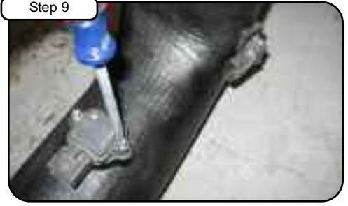
Step 9 Install MAF sensor with gasket and screws provided. Install air temp sensor with screw and gasket provided. With grommet provided, install into tube.
