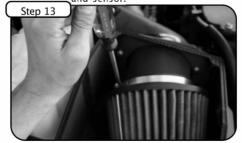
Install air filter and tighten using 5/16" nut
