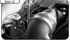
Tighten clamps @ turbo end with 5/16" nut driver. Re-connect MAF sensor harness.
