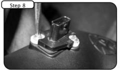
Remove MAF sensor from OE intake with T-20 torx bit. Insert MAF sensor into new tube with gasket, nylon spacer and #8-32 screws provided, spacers and gasket should be between tube and sensor.
