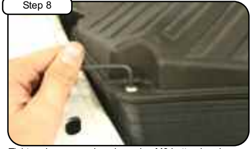
Tighten down cover housing using M6 button head screws and wavy washers.
