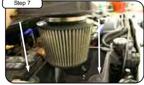
Install air filter to cover housing, tighten using 5/16" nut driver. Place cover to bottom of housing and set to position.
