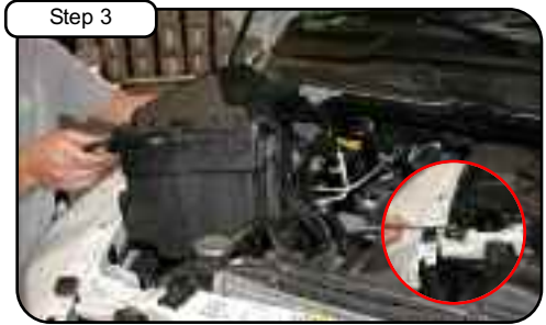
Disconnect air temp sensor. Loosen 10mm nut holding in front of air box using wrench or socket. Lift up and pull OE air box out of vehicle.
