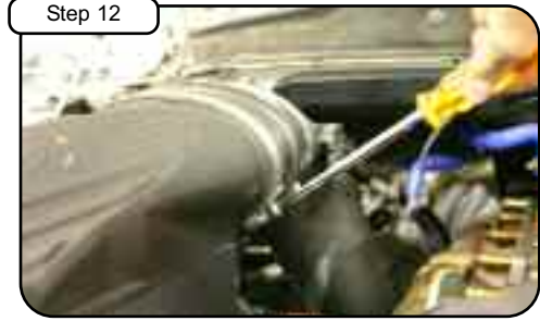
Tighten clamps at upper-cover with 5/16" nut driver.
