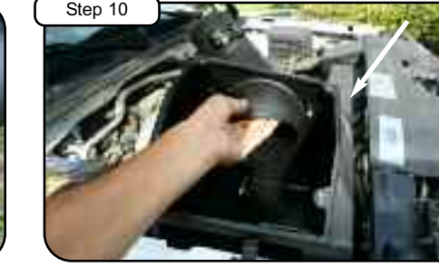
Step 10 Install housing with tube into vehicle and position.
