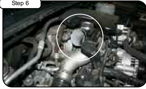
Step 6 Loosen clamp on turbo with 5/16" nut driver. Remove factory intake tube.
