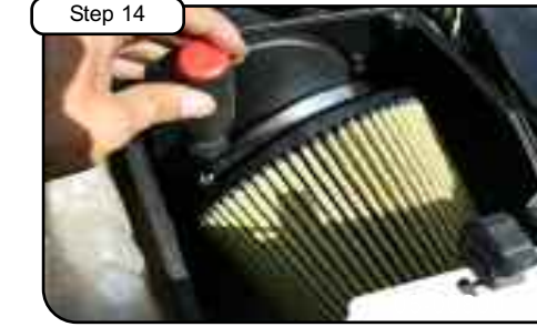
Step 14 Install air filter and tighten using 5/16" nut driver. Attach cover to housing using provided button head screws. Tighten using 5/32" allen key. Reconnect battery terminals.
