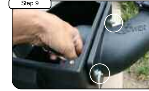
Step 9 Attach tube to outside of housing using screws, nuts and fender washers provided and tighten using 7/16" socket or wrench.
