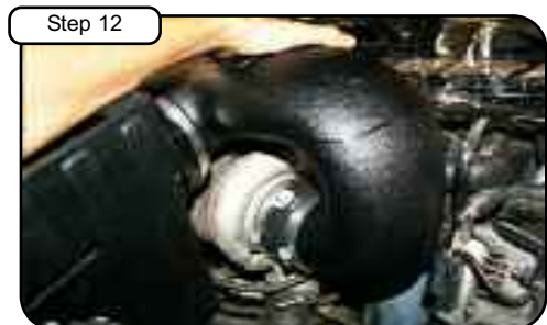
Attach 6" hump coupler with clamps provided to tube and install tube to turbo and filter adaptor. Adjust and tighten all clamps with 5/16" nut driver.
