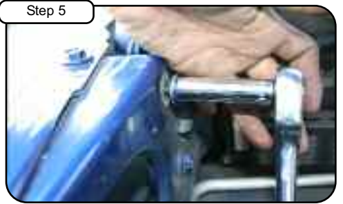
With 13mm socket or wrench remove top bolt on inner fender next to air inlet hole.
