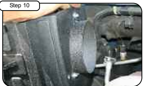
Install filter adaptor to outside of housing using supplied screws, washers, and nuts. Tighten with 7/16" socket or wrench.
