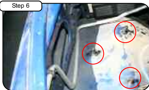
Remove plastic fittings from bolts on existing stock location mounts. Make sure 1/4-20" screw is showing.
