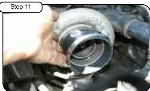
Install high temp coupler to turbo using clamps provided. Do not tighten.
