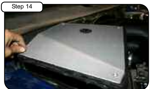
Install cover and tighten using button head screws provided. Tighten with 5/32" allen key.
