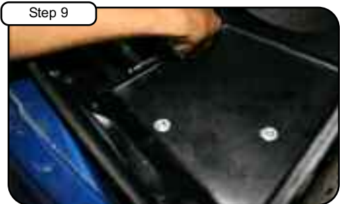
Secure housing using fender washers and nuts provided. Tighten using 7/16" socket or wrench.
