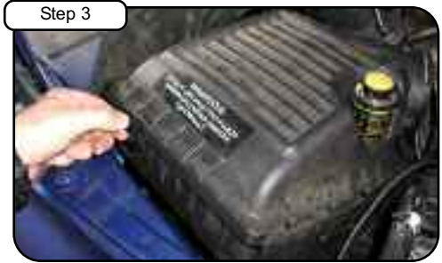
Un-clip upper half of air box and remove.
