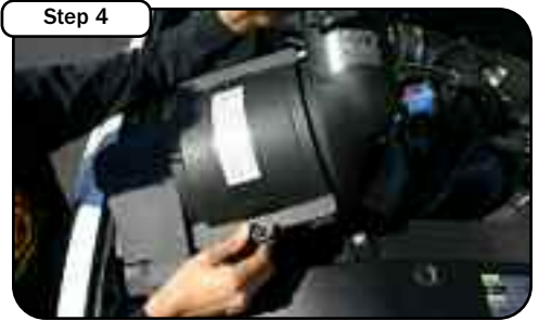
Gently pull out whole airbox. Grab from MAF area, (not directly on MAF) and pull up. It is held in place with rubber grommets. Remove the airbox mounting plate bracket.
