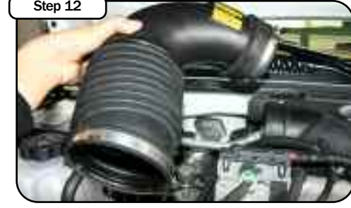
Additional steps for Stage 2 installation: With 5/16 nut driver loosen both clamps on factory tube and remove.
