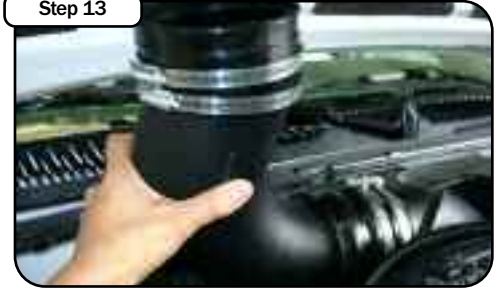
Install 4 3/4" coupler onto tube, (05-00749) using clamps provided. Install 4 1/4" end of tube into coupler. Do not tighten.
