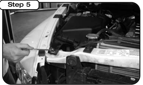
Using a 10mm wrench, remove the bolt that secures the factory airbox to the radiator bulkhead.
