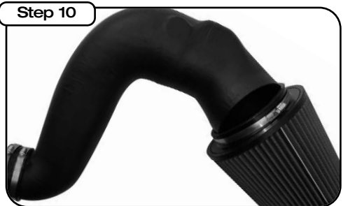
Before installing the new intake tube into the vehicle, install filter and coupler on tube ends first. Fasten the filter securely, but do not tighten coupler.
