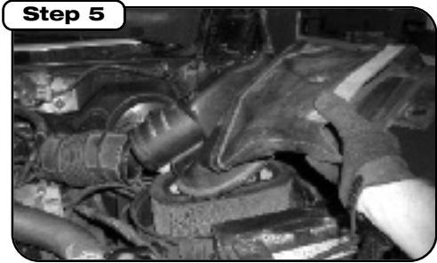
Remove top half of air box from lower half. Remove factory intake tube from factory turbo inlet elbow.
