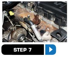
Disconnect the exhaust back-pressure tube from both the exhaust manifold and the sensor block and remove the tube. Remove the nuts holding the heat shield on the front of the exhaust manifold and remove the heat shield. Remove the bolt holding the transmission dipstick to the exhaust manifold.
