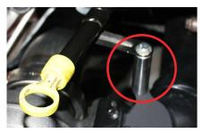
Located the supplied 3/8" double-sided studs and install them into the threaded holes on the T4 mounting flange on the HSM exhaust manifold. Slide the supplied T4 gasket onto the previously installed studs and using the supplied 3/8" nuts, install the supplied SX-E turbocharger onto the HSM exhaust manifold. Torque the nuts to 35 ft-lbs.
