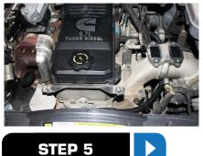
Remove the clamps from the passenger side factory intercooler pipe and remove the pipe from the vehicle.
