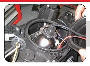
Pictured is the H7 HID bulb installed correctly in the headlight housing.
