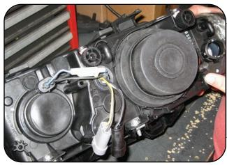
Once OEM headlights are removed from the vehicle, it will be much easier to do your HID install. Pictured are the low & high beam dust covers, this will require minimum modification in order install your H7 HIDs correctly.
