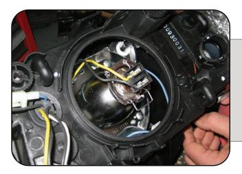
Once the low beam dust cover is removed, your low beam bulb and positive/negative connector will be exposed.
