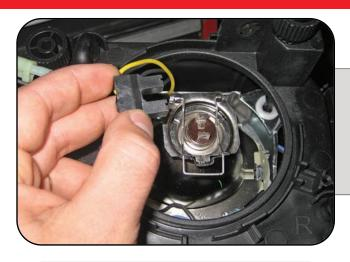
Disconnect the positive and negative female spade connector from the headlight by pulling firmly away from the low beam bulb.
