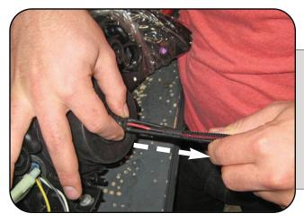
**GENTLY** pull on the wires while holding the rubber grommet firmly in place. This will eliminate any slack inside the headlight housing, giving you more wire to work with.
