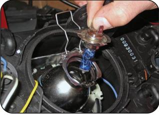
Gently remove the OEM H7 bulb out of the headlight housing.
