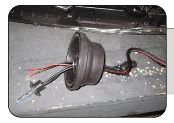
Carefully pass the H7 HID bulb and wiring through the modified low beam dust cover.
