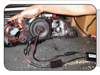
Finally, you will need to plug your OEM low beam power supply back into its' original location on the headlight housing. NOTE: Pictured is the connector for the BMW E39 5 series, plugs may vary depending on the vehicle.
