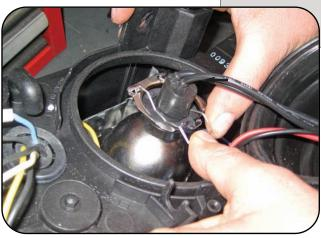
Secure the H7 HID bulb in the headlight housing by reinstalling the metal retaining clip.
