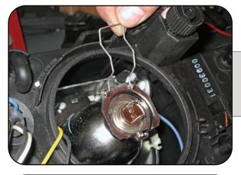
Pictured is the metal retaining clip fully unlocked.
