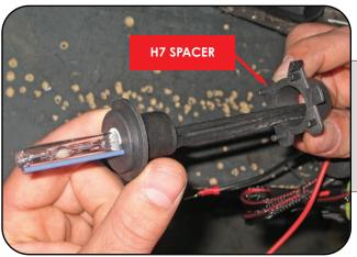
Pictured is the H7 spacer. Many cars do not need the spacer. If you do need the spacer, slide it to the base of the H7 HID bulb.
