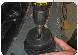
Using a drill with a Uni-bit (pictured) or a 7/8" wood spade bit drill a 7/8" hole in your low beam dust cover. This will allow you to pass the HID wiring through. The hole must be located DIRECTLY behind the bulb location.
