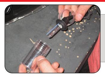
Remove the H7 HID bulb from the protective plastic casing and screw cap. Do not touch the bulb with your bare hands. If you do, be sure to clean the bulb with rubbing alcohol prior to installation.
