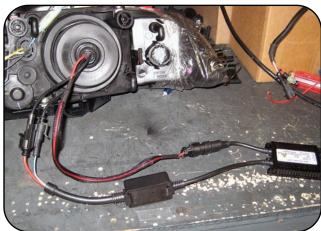
Pictured is all the wiring installed correctly.
