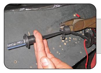
If you do not need the spacer. You can dispose of it by cutting it with wire cutters. Be careful not to cut the wires.
