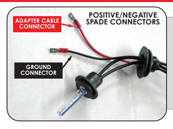
Coming through the rubber grommet on the H7 HID bulb side there will be a positive and negative spade connectors. These will be plugged into your female spade connector inside your headlight. Please observe polarity (+/-).
