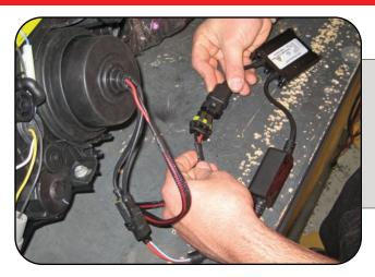
plug the 9006 connector on the adapter harness to the ballast. Mount the ballasts in a dry, flat, clean location.
