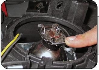
Next, pinch and release the metal retaining clips which will allows the OEM H7 low beam bulb to be removed.
