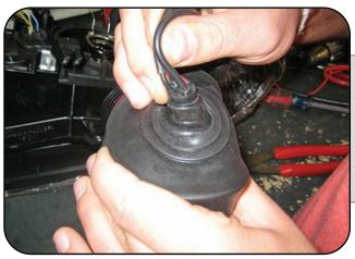
Pinch half of the rubber grommet through the 7/8" hole, sealing your low beam from the elements.
