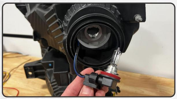
2. INSTALL THE 2STROKE 4.0 INTO THE HOUSING AND PLUG THE BULB INTO THE FACTORY WIRING
