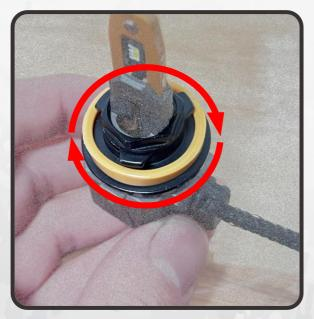
5. IF YOUR VEHICLE REQUIRES ANTI-FLICKER PWM MODULES (AVAILABLE SEPARATELY), INSTALL THE MODULE INLINE BETWEEN THE BULB AND FACTORY WIRING AS SHOWN BELOW
