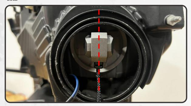
4. TO ADJUST THE ROTATION OF THE BULB, REMOVE IT FROM THE HOUSING AND USE THE PROVIDED TOOL TO LOOSEN THE NUT ON THE COLLAR. WITH THE NUT LOOSENED, ROTATE THE COLLAR TO THE DESIRED POSITION TO ACHIEVE THE DESIRED BULB ALIGNMENT. THEN, TIGHTEN DOWN THE NUT, REINSTALL THE BULB, AND CONFIRM THAT IT IS NOW CORRECTLY ORIENTED. MAKE ADDITIONAL ADJUSTMENTS IF NECESSARY
