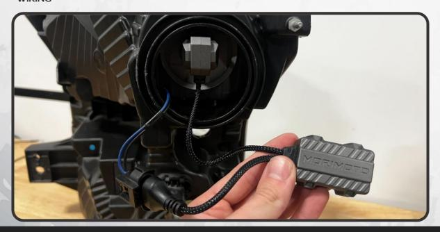
3. WITH THE BULB INSTALLED, IT SHOULD BE ORIENTED IN THE HOUSING AS SHOWN BELOW, WITH THE WIRES COMING STRAIGHT DOWN OUT OF THE BOTTOM OF THE BASE OF THE BULB
