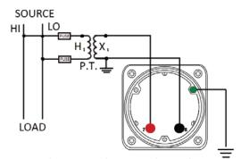
AC Voltmeter With Potential Transformer
