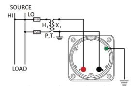
AC Voltmeter With Potential Transformer
