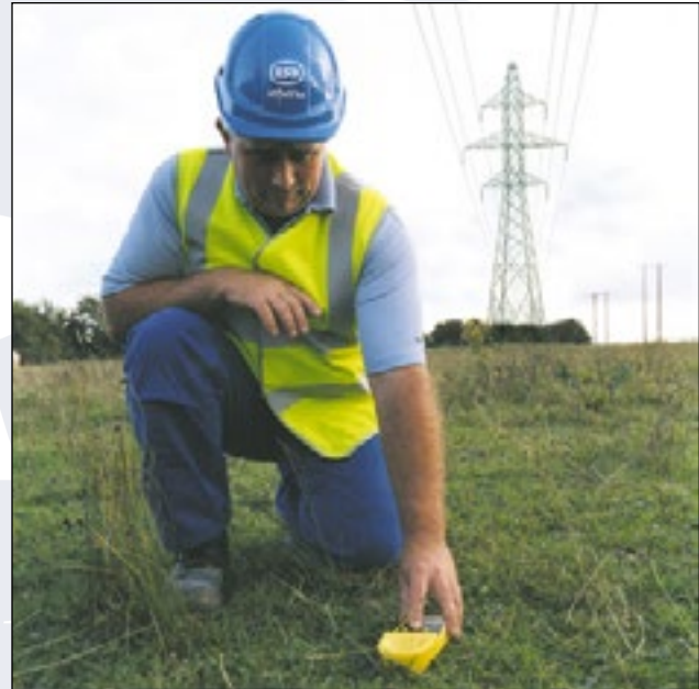
ESB employee taking a reading with cable height meter. (Photo courtesy of Suparule Systems, Ltd)
