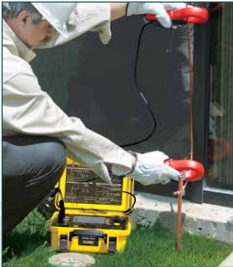
The Model 6471 provides a fast and easy way to measure the value of the earth/ground using the 2 Clamp method (no auxiliary rods needed).
