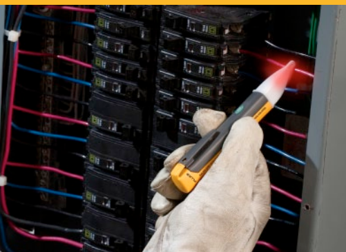
1AC-II with beeper, on-off and self test
