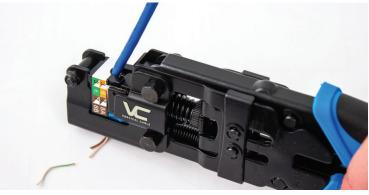
Firmly squeeze the handles together, release the handles and repeat this step to ensure a proper termination.
