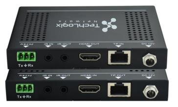
The TL-TP70-HDC is an ultra-thin extender set consisting of a transmitter (TL-TP70-HDC-T) and a receiver (TL-TP70-HDC-R). The set transmits an HDMI signal to the receiver up to 70m distance via a Cat5e/Cat6A cable. Featuring bi-directional IR and RS232, you can control your display or source using included accessories. With bi-directional PoE power, you only need to connect the power supply on one end.
