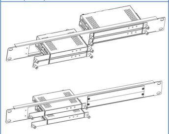
**Step 3.** Put transmitters or receivers into the slots, and then tighten the captive screws. For the empty slots, install filler plates with screws (2.5\*5mm) to cover them.
