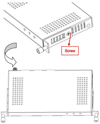
**Step 2.** Connect two Supports (1) to Twisted Pair Transmitter or Receiver (2), and fix them with screws (3\*6mm).
