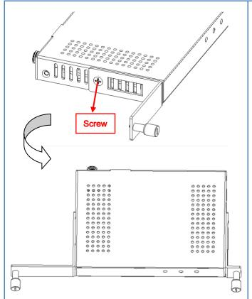
**Step 1.** Connect one Support (1) and one Support (2) to Twisted Pair Transmitter or Receiver (1), and fix them with screws (3\*6mm).
