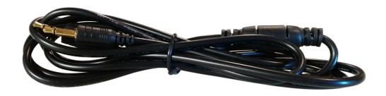
The TechLogix TL-IR-CC allows direct IR to IR connections between devices. The IR IN (TRS) connector is compatible with an IR input which provides +5V DC to the tip of the connector. The TL-IR-CC allows direct connection between the IR output of a third-party control system and a TechLogix extender. The TL-IR-CC will also allow daisy-chaining IR signals between TechLogix extenders.
