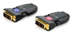
The TL-FO-DVI is a mini DVI optical fiber extender, including a transmitter and a receiver. It is compatible with HDMI video up to 4Kx2K/30Hz, and extends HDMI/DVI video up to 300m via single optical fiber cable with EDID management.
