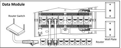
**Step 3a**: Terminate cables on the 4-Pair 110 connectors on the data module. Connect one end of a patch cord to the corresponding jack and the other end to the Ethernet router after identifying the port to activate.
