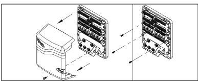
**Step 1**: Remove the screw to separate the cover from the base. Next, screw the base to a surface at a desirable indoor location using a minimum of 3 points.
