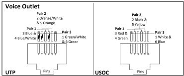
**Note**: Follow UTP or USOC wiring on 6P6C voice modular connectors to connect up to 3 phone lines per outlet.
