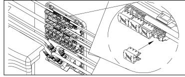
**Optional:** To protect termination wires and debris from entering 110 connectors, termination cap can be use (sold separately).
