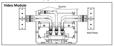
Step 3b: Attach a coaxial cable from the antenna or cable TV source to the "IN" connector on the splitter. Up to 4 TV tuners can be connected to the "OUT" connectors.
