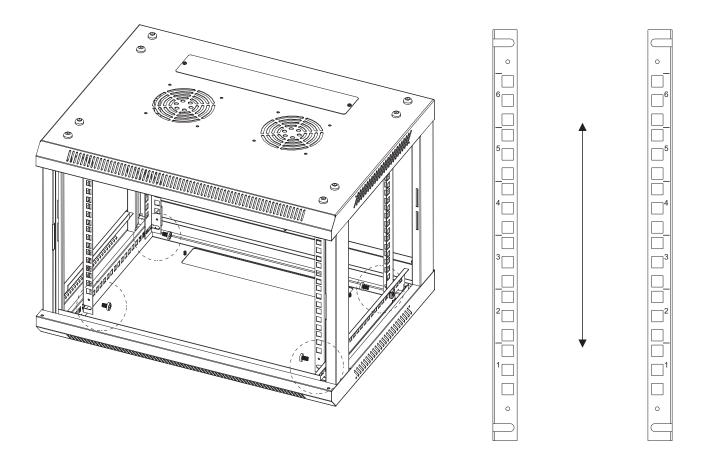
**Note:** Be sure that the rail depth is the same on both sides of the cabinet. Pay attention to the numerical unit markings on the rails to be sure they are right side up.
