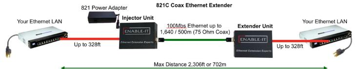
The Overview Diagram: This diagram shows the contents of the product box inside the rectangle. Devices outside the rectangle above are your equipment that can be attached.
