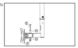
Attach the LCD mount to the bracket using the four (A) or (B) screws provided.
