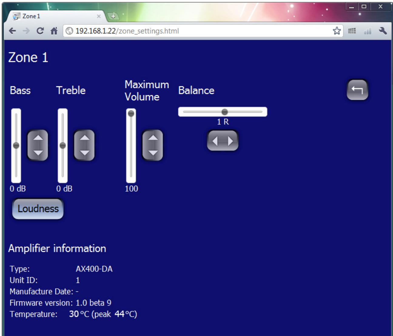
There is information displayed about the connected amplifiers Model and Unit ID and current Firmware version. The amplifier heatsink temperature is also displayed.
