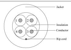
This cable is constructed by cabling together four conductors of 22 awg stranded bare copper conductors insulated with color coded polyvinyl chloride into two pairs, individually shielded. A jacket of gray colored polyvinyl chloride completes
