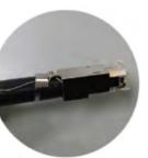
Crimp and fold down the cable holder (located on back of connector) to secure the ground wire and cable
