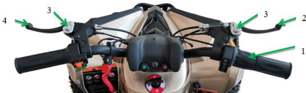
① Accelerator ② Front brake handle ③ parking braking ④ Rear brake handle
