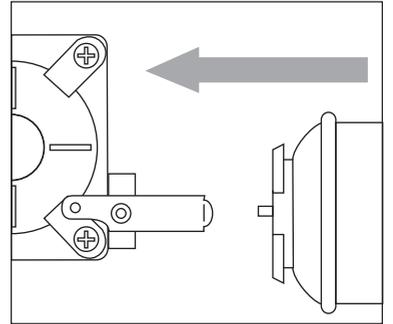
3. When you are ready to use the stove, push the cartridge lever down to the FUEL-LOCK position. If a hissing sound or gas smell is evident, check that cartridge is fitted correctly. Repeat step 2 to stop the gas leakage. **If lever is hard to push down, do not force it. Check that the cartridge is fitted correctly and the control is in the OFF position.**
