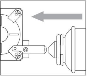
3. When you are ready to use the stove, push the cartridge lever down to the FUEL-LOCK position. If a hissing sound or gas smell is evident, check that cartridge is fitted correctly. Repeat step 2 to stop the gas leakage. **If lever is hard to push down, do not force it. Check that the cartridge is fitted correctly and the control is in the OFF position.**
