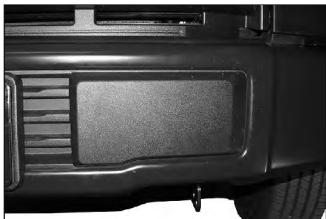
(Fig 5) Remove bumper pads to access splash guard hardware if necessary. 2015 F150 pictured
