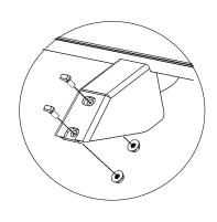
Position step tube over protruding t-bolts. From behind bracket, PUSH UP AND TURN Flange nuts (Item E) to engage t-bolts in slots and tighten.
