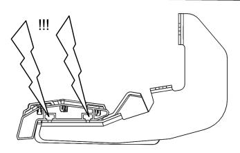
CAUTION!! - Be sure to engage t-bolts into slots. Push UP and TURN to tighten. Verify t-bolts are engaged before torquing fasteners.
