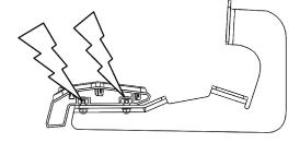
CAUTION!! - Be sure to engage tbolts into slots. Push UP and TURN to tighten. Verify t-bolts are engaged before torquing fasteners.
