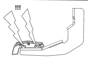
CAUTION!! - Be sure to engage t-bolts into slots. Push UP and TURN to tighten. Verify t-bolts are engaged before torquing fasteners.
