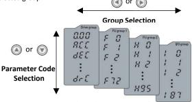
Any of the above parameters and monitors settings can be accessed by pressing the ENT key.
