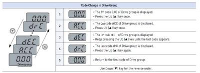
Pressing the LEFT or RIGHT arrows will move through the different parameter groups. While the UP and DN arrows will navigate through the different parameter code #'s in the selected group.
