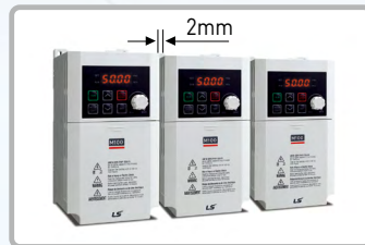
Side-by-side Installation (2mm between drives)
