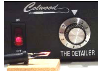
"K" Tip glowing with Detailer set to max power
