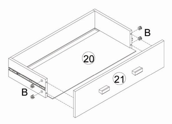
Slide Part 20 into the sides, attach part 21 to the sides of the drawer using 4 x B.
