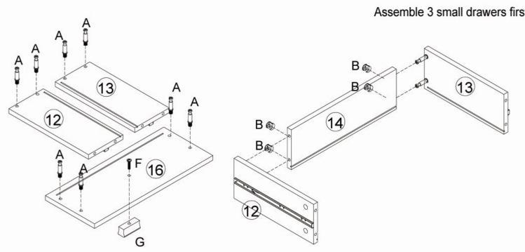
Screw in 8 x A locking pins to Part 12,Part 13 and Part 16.Using 1 x F handle screw, screw on 1 x G handle.
