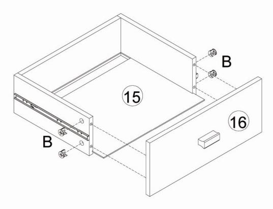
Slide Part 15 into the sides, attach part 16 to the sides of the drawer using 4 x B.
