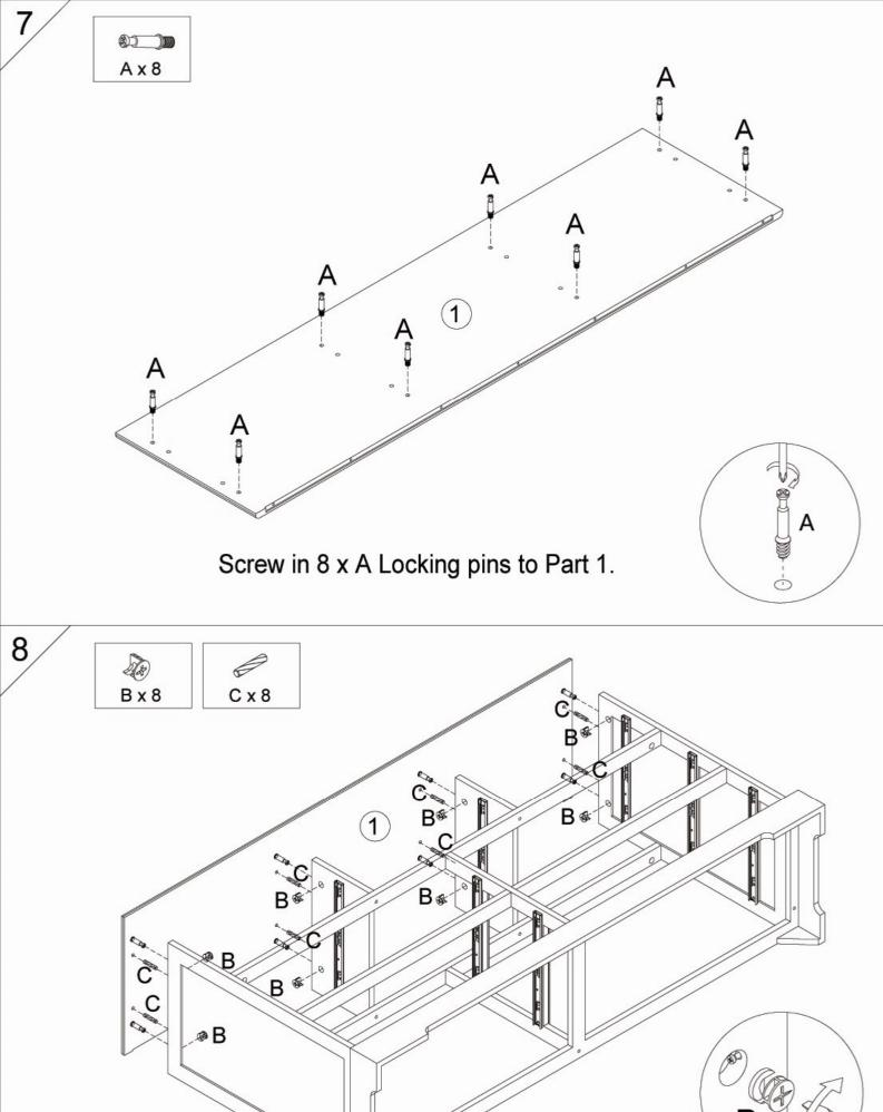
To attach the top of the chest to the base using 8 x B and 8 x C.
