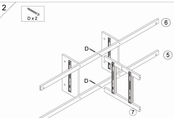
Connect Part 7 to Part 5 and Part 6 using 2 x D.
