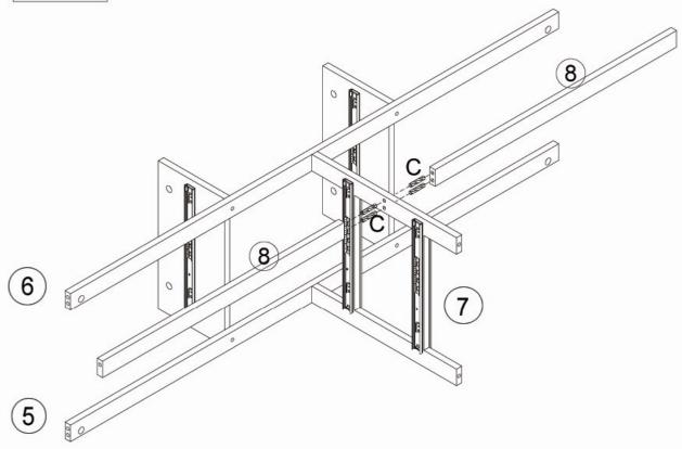
Connect 2 x Part 8 to Part 7 using 4 x C.
